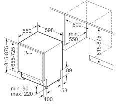
measurements in mm
